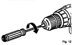
Insert allen wrench in chuck and tighten chuck jaws securely. Tap sharply with a mallet in a counterclockwise direction. This will loosen chuck on the spindle. It can now be unscrewed by hand. See Figure 13.
